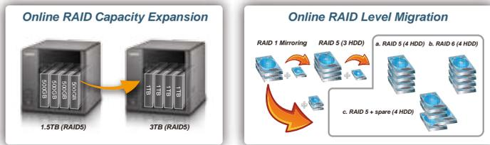
The TS-410 supports online RAID capacity expansion for expanding the storage capacity of the RAID configuration and online RAID level migration for upgrading the disk configuration to higher RAID level.
