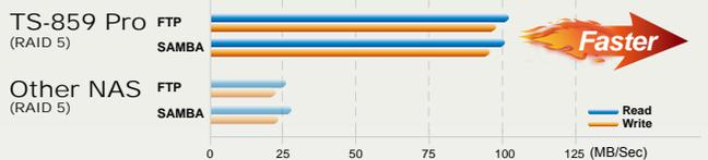
\* FTP/SAMBA Testing Environment: Intel Core2 Quad CPU Q8300 2.50GHz/ 4GB DDRII RAM, WD640AAKS 640GB, Windows 7 Enterprise 32 Bits, Intel PRO 1000 FT Dual Port Server Adapter 82571
